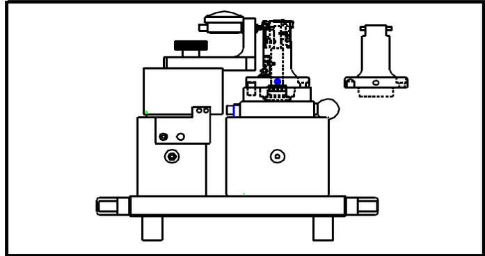
**M**aster Tool was asked to design and quote a boring system for a large compressor manufacturer. The operation was the finish machining of the cylinder bores for a series of six (6) different cast iron compressor housings.
